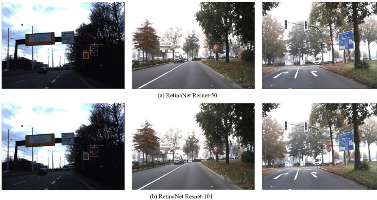
Figure 4: Examples of detections from two different models on a road with tiny, medium, and large traffic signs of varied sizes. All detections under these circumstances are precise. The third image from A, B, and C only depicts three traffic signals, yet one is still obscured.
